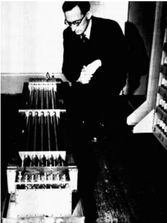
(b) Mercury delay lines or “long tanks” for the main memory, with M. V. Wilkes looking on. The battery of 16 tanks shown here had a capacity of 512 words - the equivalent of a little over 1 Kilobyte.
